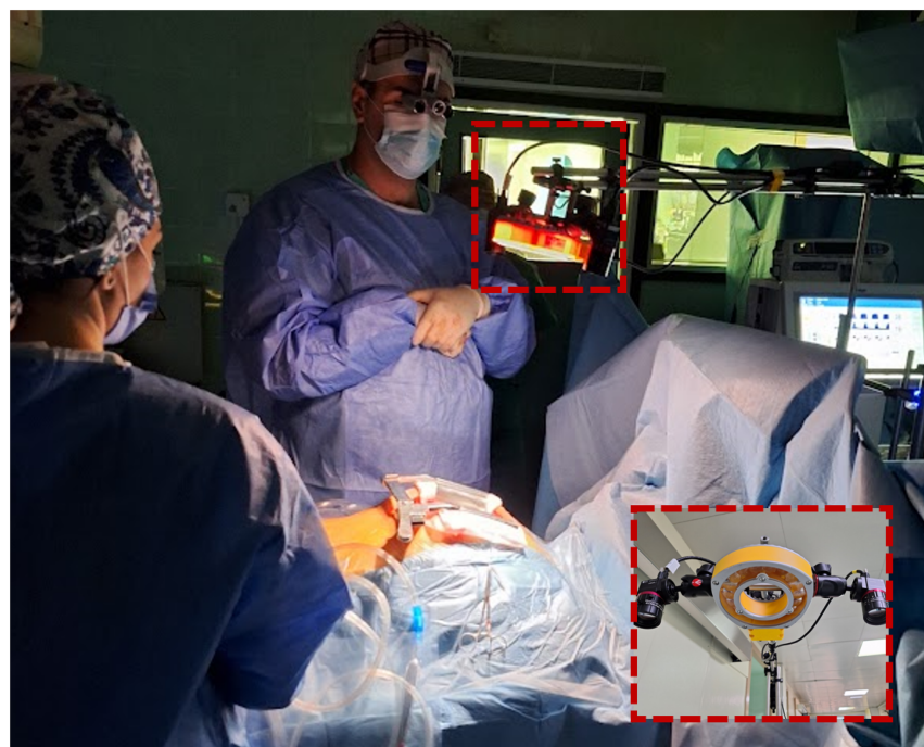
Fig. 2 Multispectral imaging system consists of an LED light source and two snapshot cameras. The system is mounted directly above the exposed heart during open surgery.
