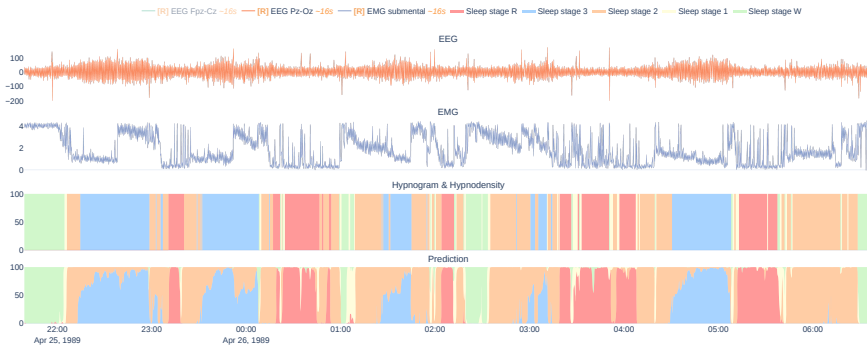
Figure 2.4: Sleep stage classification example, demonstrating the joined visualization of raw sensor data with probabilistic predictions. The first two rows show the raw data, i.e., EEG signals which are sampled at 100Hz, and an EMG signal which is sampled at 1Hz, respectively. The third row shows the sleep stages, also called a hypnogram on the right y-axis (black line), and the hypnodensity, i.e., a probabilistic hypnogram, on the left y-axis. The final row shows probabilistic hypnodensity predictions of a machine learning pipeline, empowered by tsflx [31].
