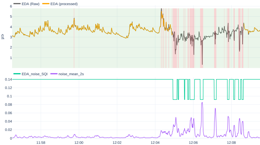
Figure 6.10: Skin conductance signal processing to discern valid and invalid regions and the resulting processed signal. Note: The figure consists of two vertically stacked subplots that share the same x-axis. The upper subplot displays the raw EDA signal depicted by the gray line, with valid and invalid SQI regions distinguished by green and red backgrounds, respectively. The processed EDA data is illustrated by an orange line. Remark that there is no one-on-one relationship between the processed EDA data and the valid regions. This is because the duration and frequency of these invalid regions affect the eventual retention of the raw EDA signal. Specifically, brief and infrequent invalid segments, like those until 12h05, can be effectively imputed using interpolation, resulting in no data exclusion in the processed EDA signal. Conversely, as the frequency and/or duration of invalid segments increases, evidenced between 12h05 and 12h06, successful interpolation is compromised, resulting in disregarding these invalid regions. Moreover, processed EDA segments, but shorter than 60 seconds (e.g., valid segments between 12h06 and 12h08), are excluded given their limited analytical utility. The lower subplot elucidates the components of the skin conductance SQI. In alignment with the non-wear detection pipeline, multiple sub-SQIs are utilized. The noise amplitude of the EDA, averaged over a two-second window, is delineated by a purple line. This signal is thresholded to determine the noise sub-SQI, marked by the green line.
